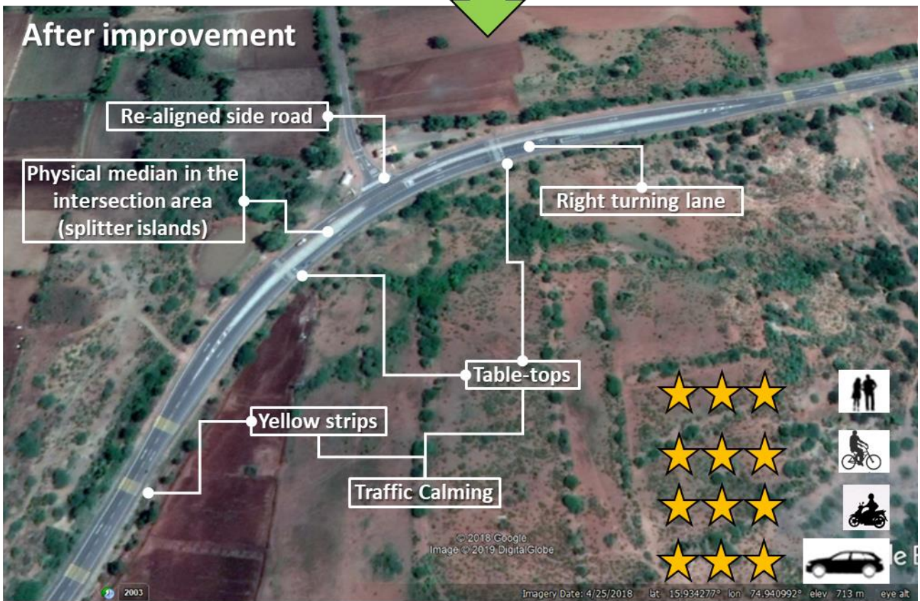
Figure 16 Before and after Improvement image of intersection, Km 46.9
