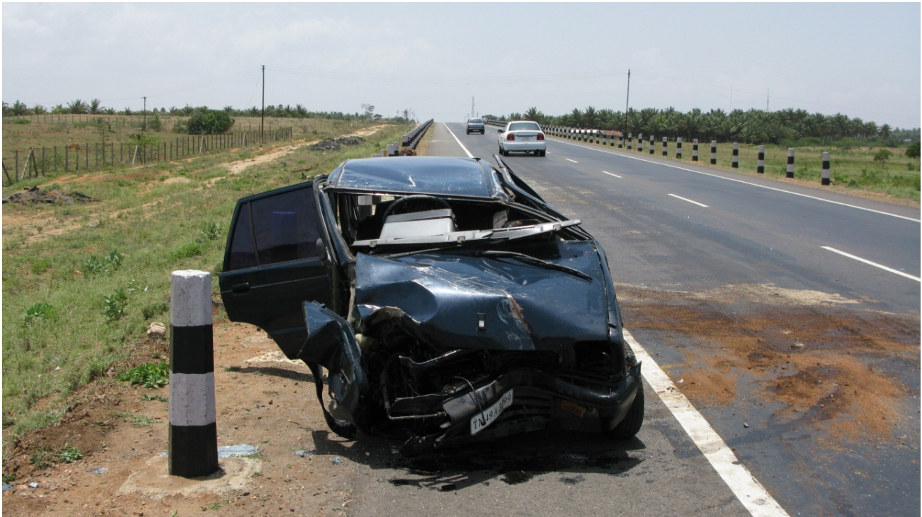
Figure 5 Result of a motor vehicle collision with pre-cast concrete guard post
